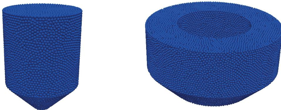
(a) HTR-10: cylindrical core geometry (b) PBMR-400: annular core geometry
