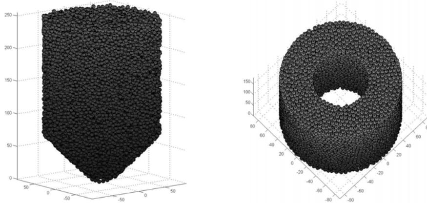
(a) Cylindrical core with conic bottom (b) Annular core
