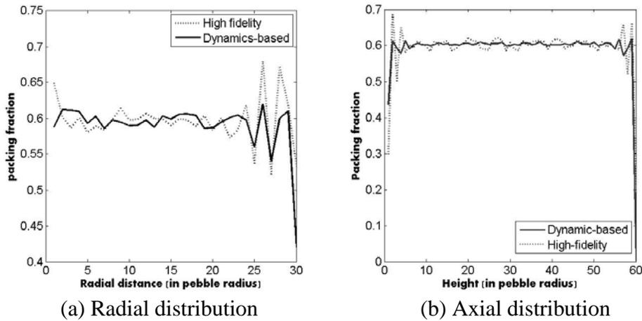
Figure 2: Radial and axial packing fraction distributions
