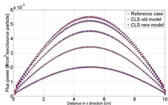
(b) Flux distribution comparisons over cells located at Y=1 (lowest curves), 2, 3, 4, and 5 (highest curves) cm
