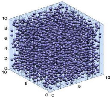
Fig. 1. Fuel particles packed in a cubic container.
