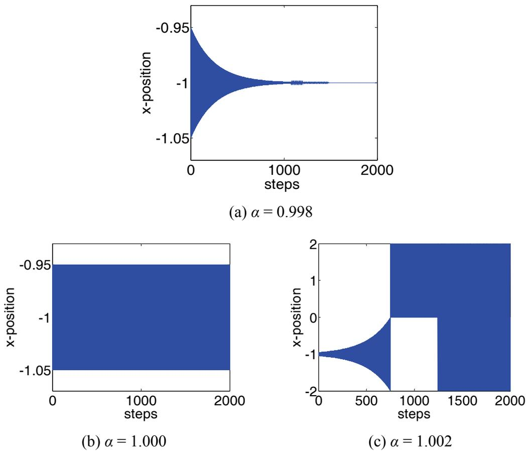
**Fig. 5.** Position history of sphere 1 under PBC. The initial perturbation is  $\delta_0=0.1$  and the initial gamma value is 0.5.
