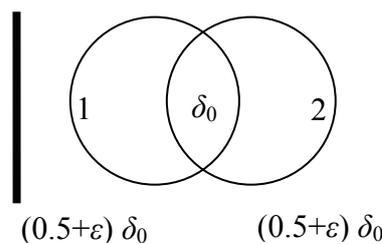
**Fig. 11.** 1-D loose packing with system width  $4r - \delta_0$ .
