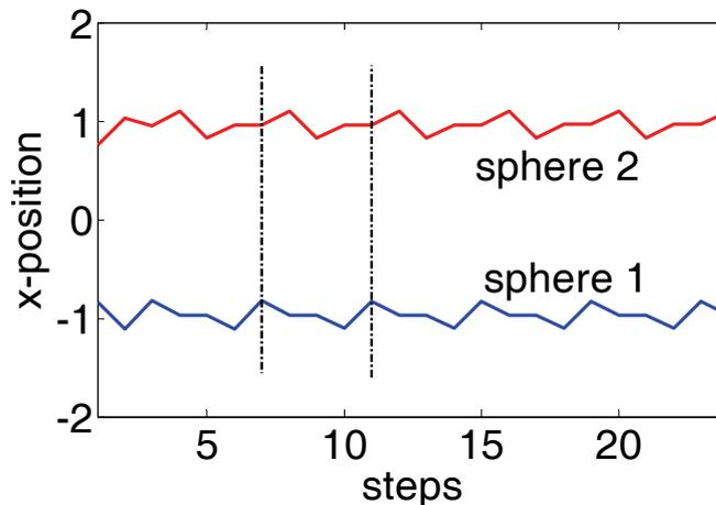
(b) Motion mode B: four-stage cycles. Each sphere experiences a four type of overlaps in each cycle but with different sequence. One sphere experiences: sphere-to-sphere overlap (1) -> sphere-to-wall overlap (2) -> sphere-to-sphere overlap (3) -> overlap free (4) ->
