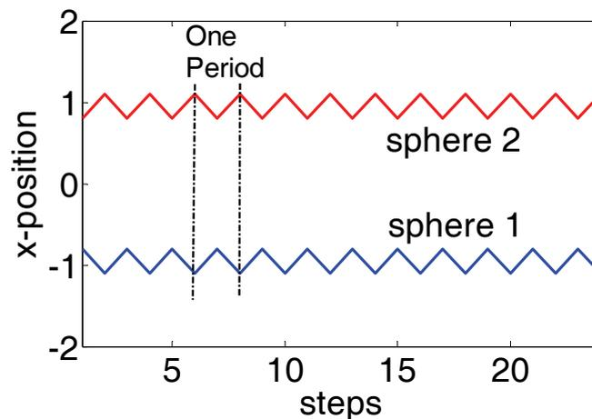
(a) Motion mode A: 2-stage cycles. Two spheres are moved always in the opposite directions at each iteration step due to the sphere-to-sphere overlap and sphere-to-wall overlap that appear alternately. Each sphere experiences the same type of overlap at each iteration step. The positions of each sphere are plotted as a function of iteration step. The figure is based on the numerical calculation with an initial perturbation  $\delta_0=0.4$  and an initial gamma value 0.5.
