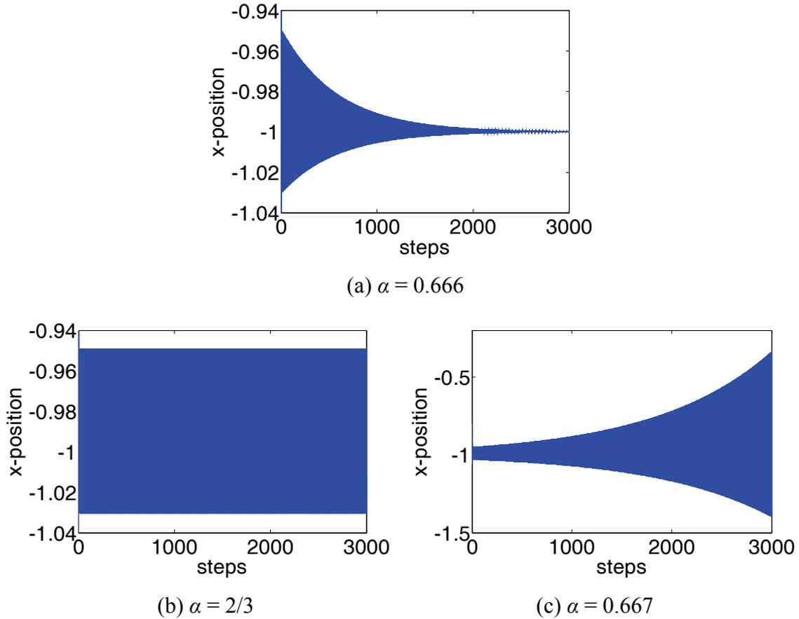
**Fig. 4.** Motion of Sphere 1 with respect to different  $\alpha$  (asymmetric initial condition under FBC). The initial perturbation is  $\delta_0=0.1$  and the initial gamma value is 0.5.
