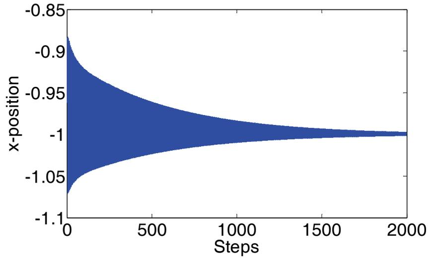
(a) x-position history of sphere 1: Fixed boundary condition,  $\alpha=0.666$ ,  $\delta_0=0.1r$  and the algorithm is convergent
