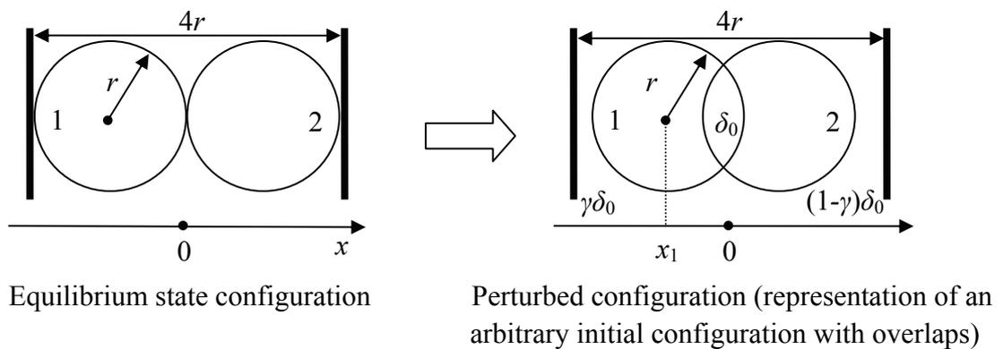
(a) Close packing of two spheres in a 1-D system with fixed boundary condition, representing the smallest 1-D packing system
