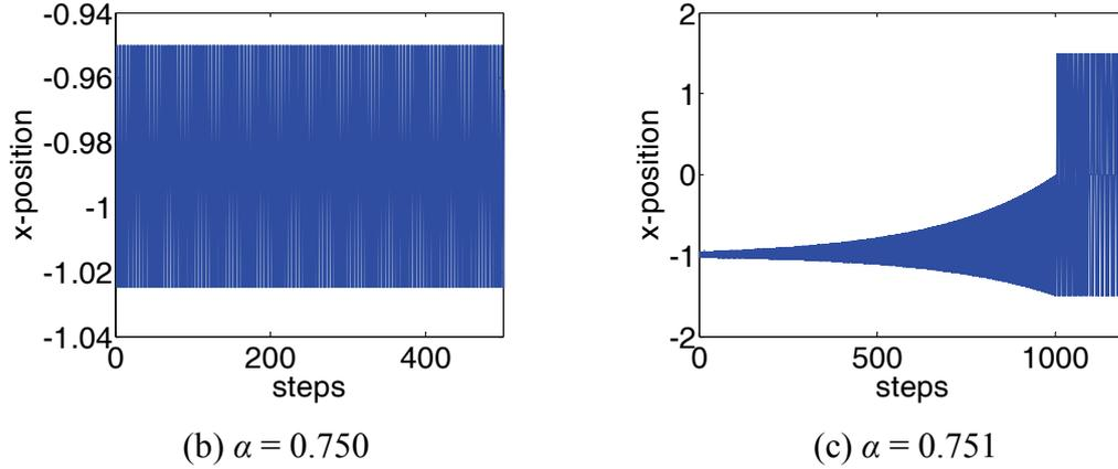
**Fig. 3.** The motion of Sphere 1 with respect to different  $\alpha$  (symmetric initial condition under FBC). The initial perturbation is  $\delta_0=0.1$  and the initial gamma value is 0.5.
