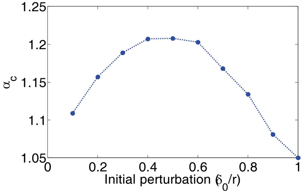
(a) Critical step size as a function of initial perturbation magnitude at the fixed perturbation direction of  $d_1=135$  degree
