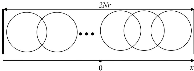
(a) geometry of N-sphere 1-D packing under FBC
