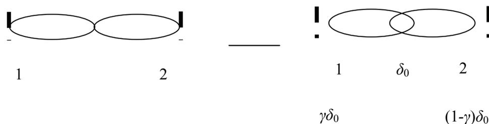
(b) Close packing of two spheres in a 1-D system with periodic boundary condition, representing the largest 1-D packing system
