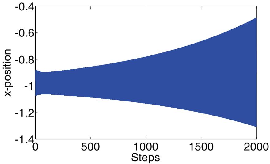
(b) x-position history of sphere 1: Fixed boundary condition,  $\alpha=0.667$ ,  $\delta_0=0.1r$  and the algorithm is divergent
