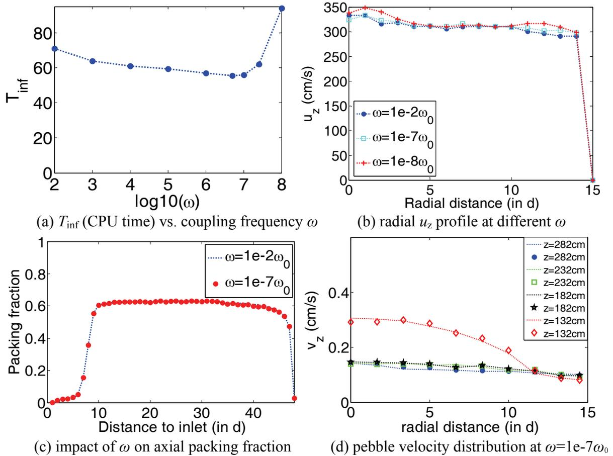
Figure 7. Impact of coupling frequency  $\omega$  on computation efficiency and accuracy
