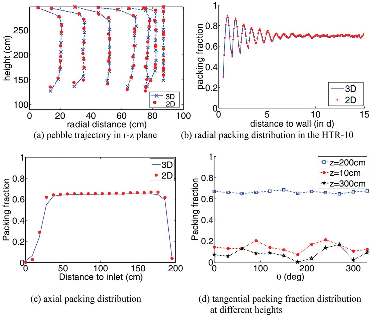
Figure 4. Pebble flow comparison of pebble trajectory and packing distribution between 2D and 3D simulation
