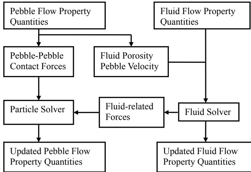
Figure 1. 3D-DEM/3D-CFD schematics
