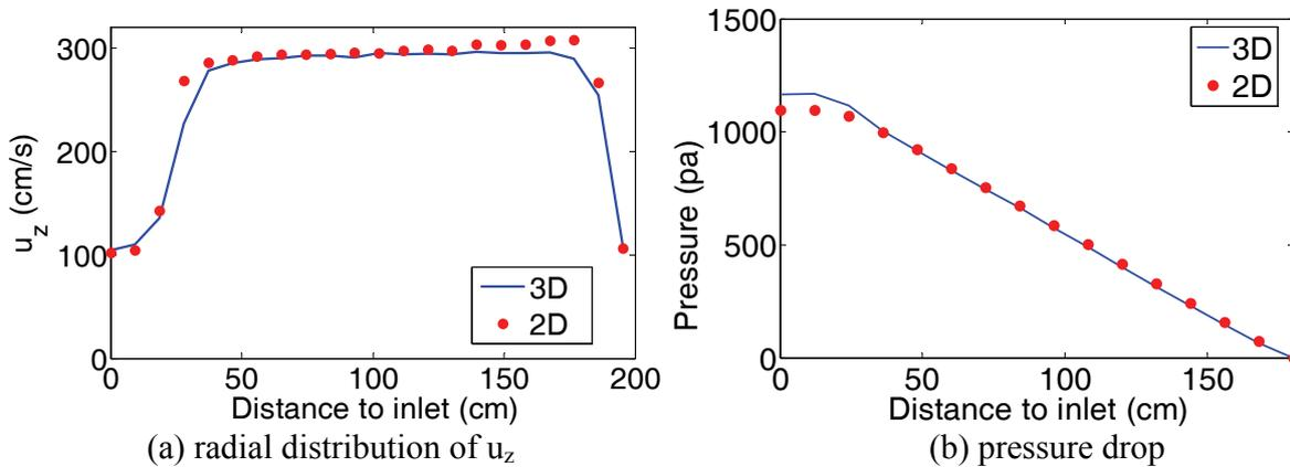
Figure 5. Comparison of z-component coolant flow velocity and pressure drop between 2-D and 3-D simulations
