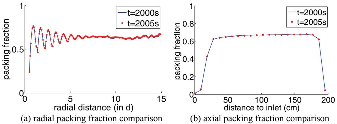
Figure 3. Comparison of packing fraction distribution at steady state between two simulation times
