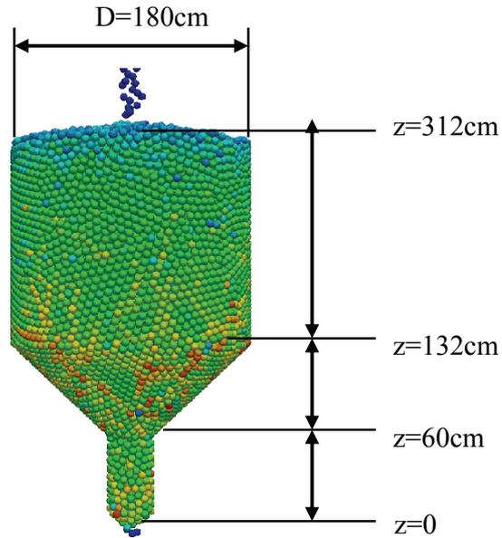
Figure 2. Reactor geometry and snapshot during pebble recirculation
