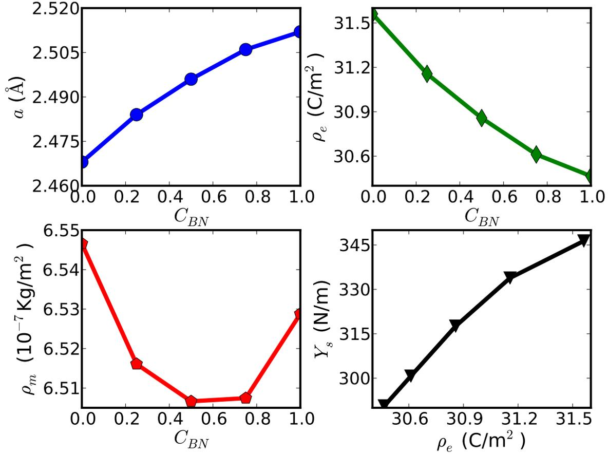
**Figure 3.** Lattice constants  $a$ , electronic charge density  $\rho_e$  and mass density  $\rho_m$  as a function of  $h$ -BN concentrations  $C_{BN}$ . The in-plane stiffness  $Y_s$  varied with electronic charge density is plotted.
