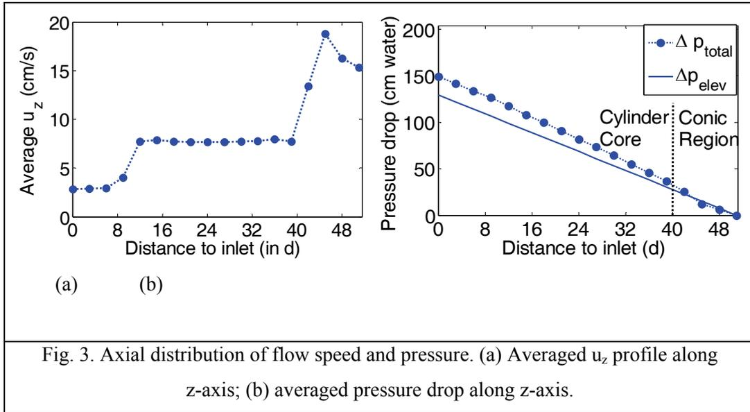
Fig. 3. Axial distribution of flow speed and pressure. (a) Averaged  $u_z$  profile along  $z$ -axis; (b) averaged pressure drop along  $z$ -axis.
