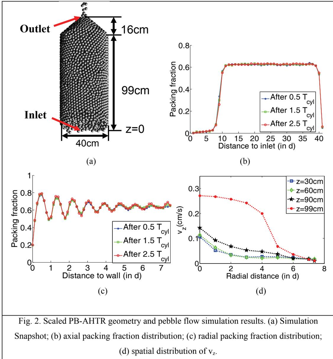
Fig. 2. Scaled PB-AHTR geometry and pebble flow simulation results. (a) Simulation Snapshot; (b) axial packing fraction distribution; (c) radial packing fraction distribution; (d) spatial distribution of  $v_z$ .
