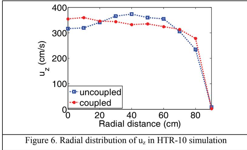
Figure 6. Radial distribution of  $u_z$  in HTR-10 simulation
