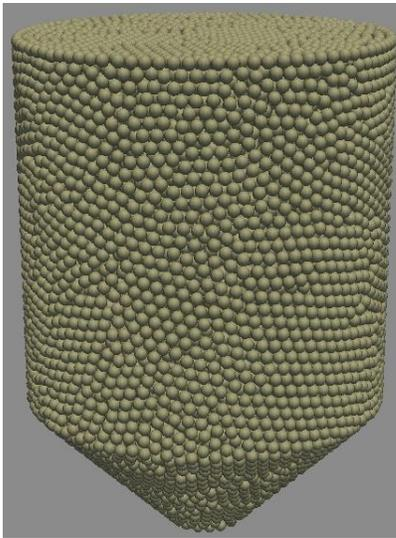
(a) HTR-10: cylindrical core geometry
