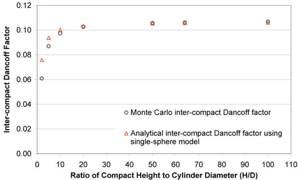
Fig. 12. Comparisons between analytical and Monte Carlo average intercompact Dancoff factors at volume packing fraction 28.92% for finite height compacts.
