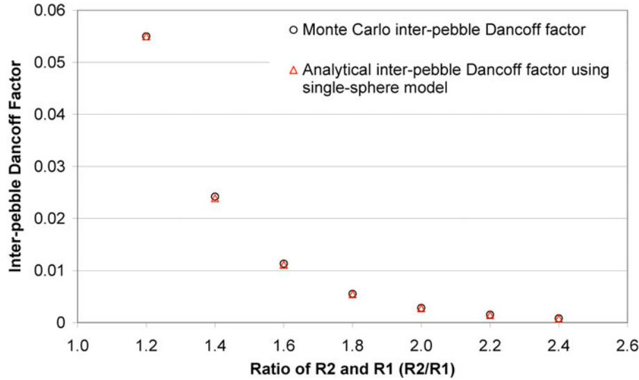
Fig. 10. Comparisons between analytical and Monte Carlo average interpebble Dancoff factors at volume packing fraction 5.76%.
