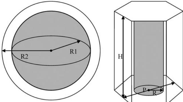
Fig. 5. Fuel pebble and fuel compact cells in Monte Carlo simulation.
