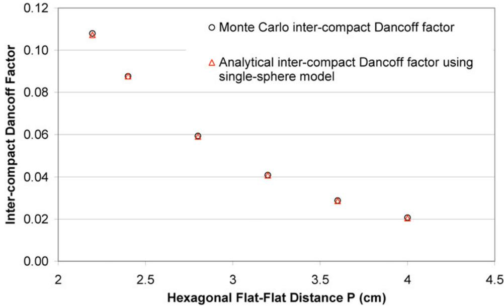
Fig. 11. Comparisons between analytical and Monte Carlo average intercompact Dancoff factors at volume packing fraction 28.92% for infinite height compacts.
