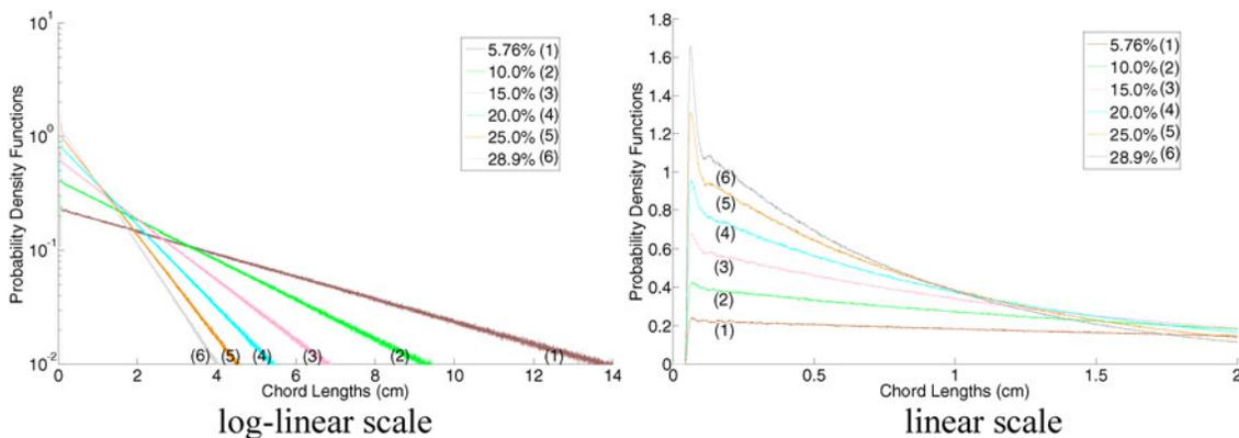
Fig. 2. Chord length PDFs between two fuel kernels.
