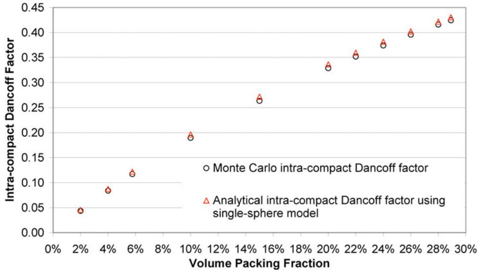
Fig. 7. Comparison between analytical and Monte Carlo average intracompact Dancoff factors for infinite height compacts.
