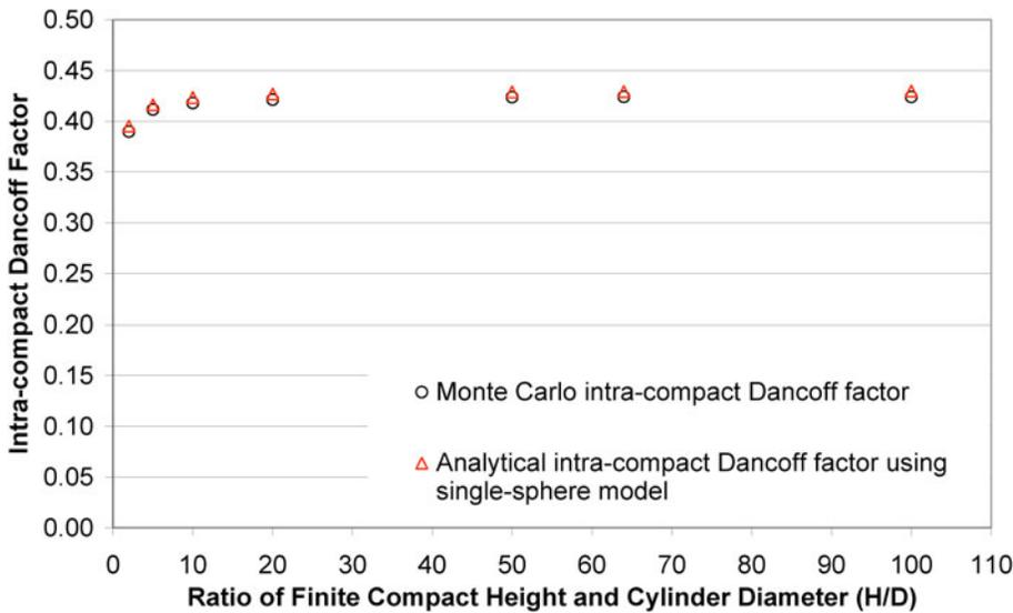
Fig. 8. Comparisons between analytical and Monte Carlo average intracompact Dancoff factors for finite height compacts.
