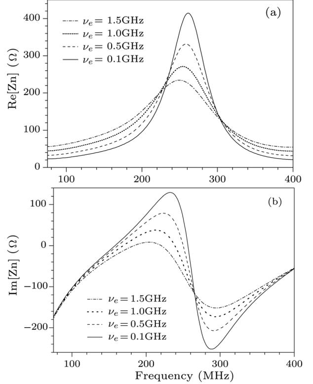
**Fig. 4.** (a) Real part of input impedances of plasma antenna with  $\nu_e = 0.1, 0.5, 1.0, 1.5$  GHz. (b) Imaginary part of input impedances of plasma antenna with  $\nu_e = 0.1, 0.5, 1.0, 1.5$  GHz. The plasma frequency is 5 GHz, the copper antenna and plasma antenna are with the same size.
