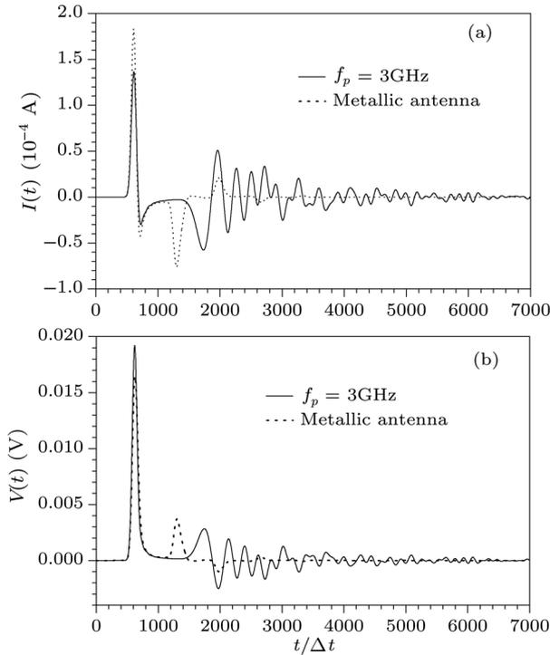
**Fig. 2.**  $V(t)$  of metal antenna and plasma antenna with  $f_p = 3$  GHz excited by a 1 V Gaussian pulse. (b)  $I(t)$  of metal antenna and plasma antenna with  $f_p = 3$  GHz excited by a 1 V Gaussian pulse.
