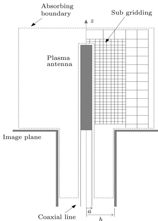
**Fig. 1.** FDTD geometry of plasma antenna fed through a coaxial transmission line.
