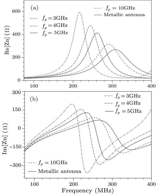
**Fig. 3.** (a) Real part of input impedances of metallic antenna and plasma antenna with  $f_p = 3, 4, 5, 10$  GHz. (b) Imaginary part of input impedances of copper antenna and plasma antenna with  $f_p = 3, 4, 5, 10$  GHz. The collision frequency is 150 MHz, the copper antenna and plasma antenna are with the same size.
