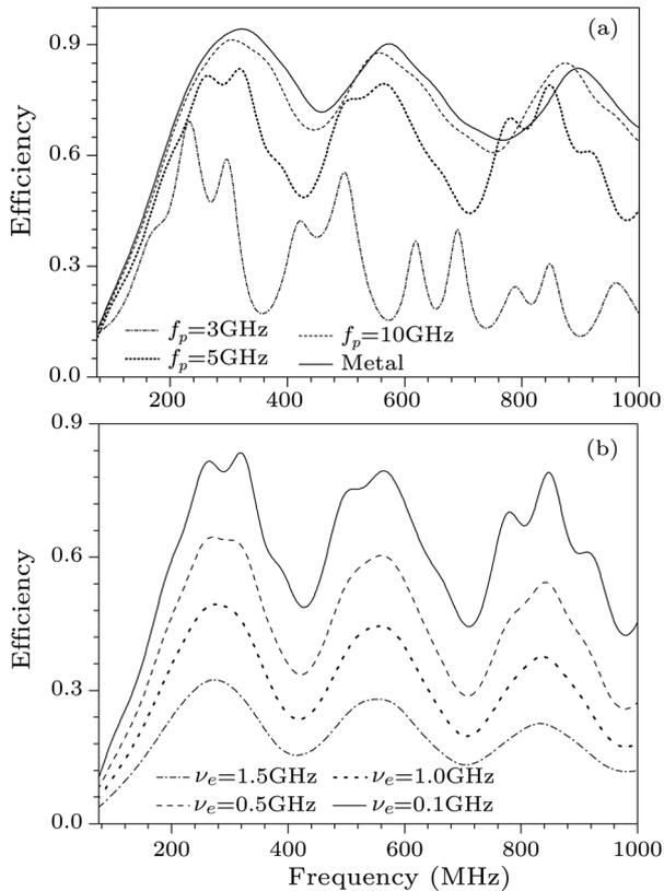
**Fig. 5.** (a) Radiation efficiency of copper antenna and plasma antenna with  $f_p = 3, 5, 10$  GHz and  $\nu_e = 150$  MHz. (b) Radiation efficiency of plasma antenna with  $\nu_e = 0.1, 0.5, 1.0, 1.5$  GHz and  $f_p = 5$  GHz.
